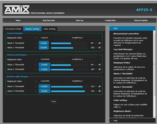
This page allows to configure for each of the three displays the value of weighting A or C and the value of Leq 1s, 1min, 5min, 10min, 15min or 60min.
