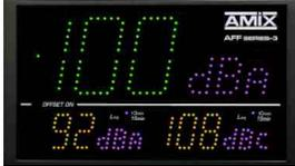
*L<sub>Aeq</sub> and L<sub>Ceq</sub> have exceeded the first threshold*
